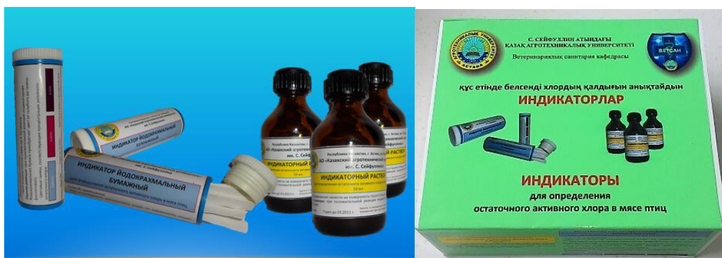
Figure 4 – The developed indicators to detect residual active chlorine in poultry meat
